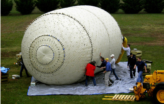
Engineers in West Virginia, financed by the Department of Homeland Security, test an inflatable plug to block flooding in transit tunnels. Photo: The New York Times , 21 November 2012.
